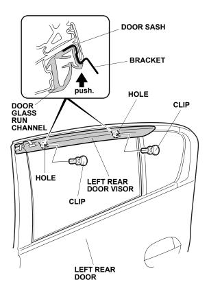
18. Adjust the left rear door visor to the position shown.
