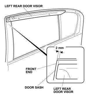
19. While holding the door visor firmly in position, remove the adhesive backing. Use your finger to push up each bracket so there is no gap between the brackets and the door sash.
