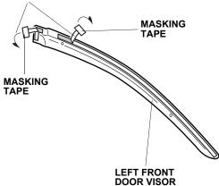
7. Align the clip holes in the visor with the bracket holes, and install two clips. There should be no clearance between the brackets and the door sash.
