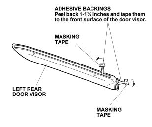
17. Align the clip holes in the visor with the bracket holes, and install two clips. There should be no clearance between the brackets and the door sash.
