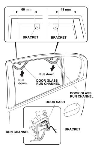
13. Install two brackets between the door sash and the run channel at the measurements shown. Then seat the run channel properly around the brackets.
