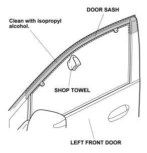
5. Remove the adhesive backing from the seal, and attach it to the door sash.
