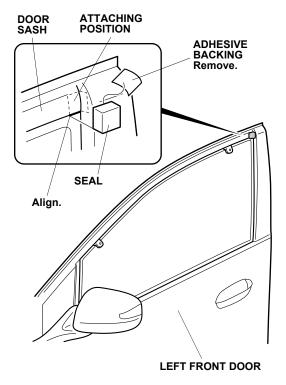
6. Peel back approximately 1-1½ inches of adhesive backing from each adhesive strip, and tape the ends to the front surface of the left front door visor.
