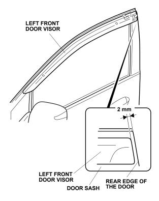
9. While holding the door visor firmly in position, remove the adhesive backings. Use your finger to push up each bracket so there is no gap between the bracket and the door sash.
